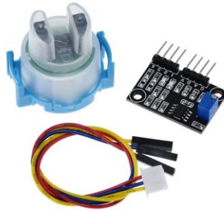
Gambar 4. Sensor Turbidity TS-300B (Sumber: innovatorsguru.com )
